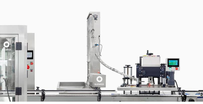
Compact bottling station from Bluewater efficiently fills, labels, caps and washes re-useable water bottles for use in hotels and restaurants, spelling an end for polluting throwaway bottles
