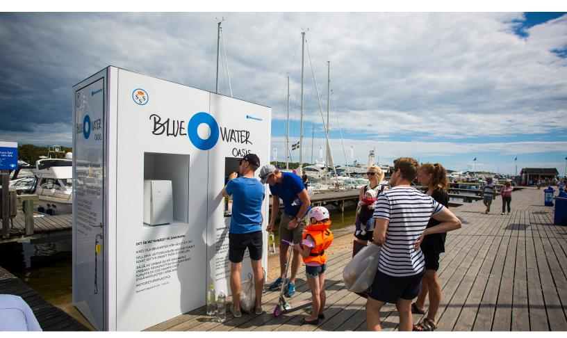
The Bluewater Oasis hydration station pumps water directly from the Baltic Sea and turns it into on-demand fresh drinking water, delivering up to 5.7 liters per minute.
