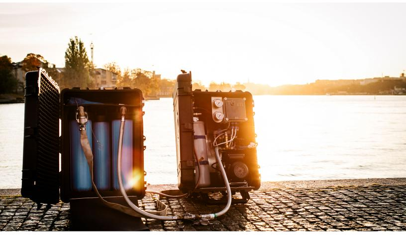
Bluewater disaster relief hydration solution features sediment filters that capture particles down to 5 microns and a unique Bluewater reverse osmosis (RO) membrane that eliminates microscopic particles (Credit: Alexander Bello)
