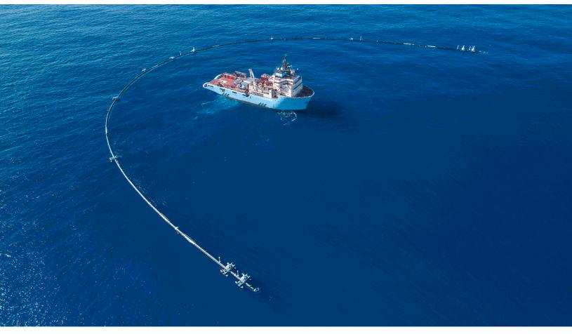
A long U-shaped pipe stretching 600 meters will capture ocean plastic waste that will end up being recycled into new products (Credit: The Ocean Cleanup)
